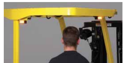
FL36VA lighthouse shown mounted in various locations on a typical forklift for safety visibility when in operation.
